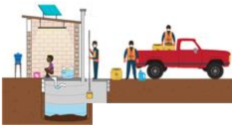
Figure 16: Lined pit latrine with emptying
