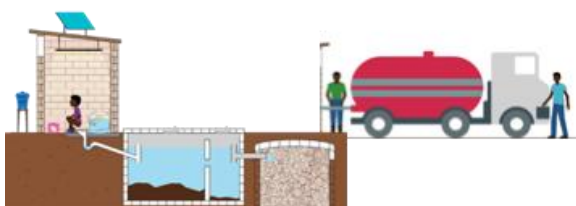
Figure 13: Individual septic tank
